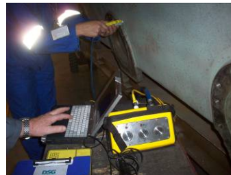
Fig 1b: ACFM in use on CR2 MBT Wheelstation
