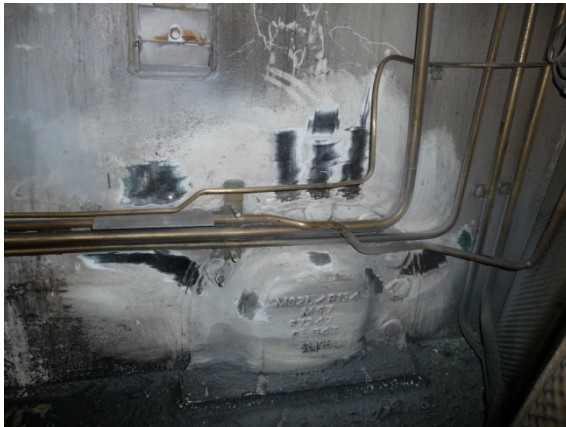
Fig 6-Wheelstation No. 5 marked up for sensors Fig 7- Electrodes (studs) being welded in place
