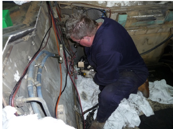
Fig 6-Wheelstation No. 5 marked up for sensors Fig 7- Electrodes (studs) being welded in place
